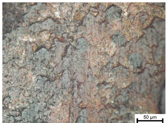
Figure 12. Aspect of the wear cap inner surface after 20 min. testing time in the ductile cast iron sample borided for 2 hours and air cooled. Sliding distance: 640 m
